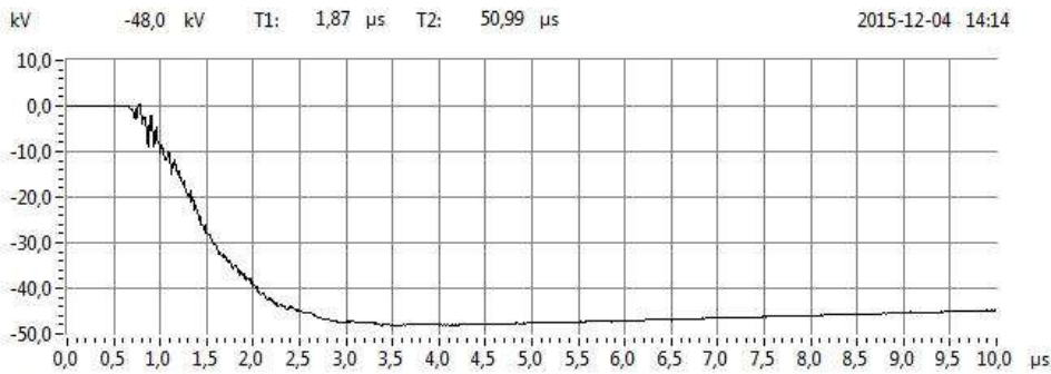
Fig. 13: Waveshape 72124900 SC loop Yellow -50% test voltage
