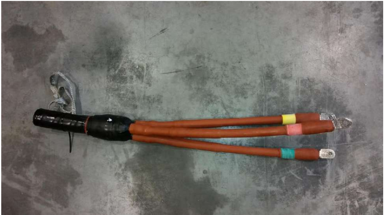
Indoor termination humidity sample
