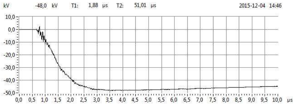
Fig. 21: Waveshape 72124900 SC loop Green -50% test voltage
