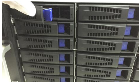
Figure 2. 7 Push the HDD Dummy into Slot
