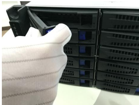
Figure 2. 3 Pull out the HDD Dummy
