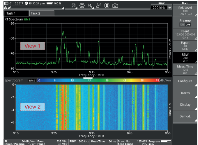
Fig. 2. RT Spectrum view (View 1) and Spectrogram view (View 1) in a task (Task 2)
