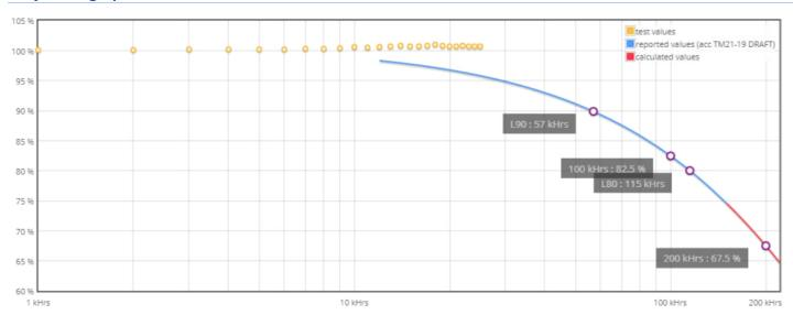
LxB50 results according to LM-80 and TM21-19 DRAFT procedures and norms.
