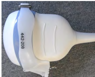
Figure 11-46 Mounting the Biopsy Needle Guide to the 4D Probe
