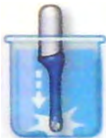
Figure 11-12 Carefully suspend probe to avoid damage to the acoustic lens
