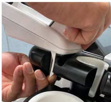
Figure 3-5 Pull the claw to remove
