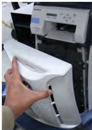
Figure 12-12 Remove the front cover
