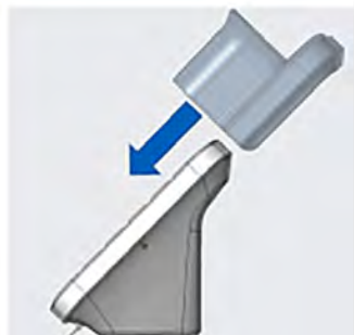
Figure 13-161 Install Probe Holder on Charger
