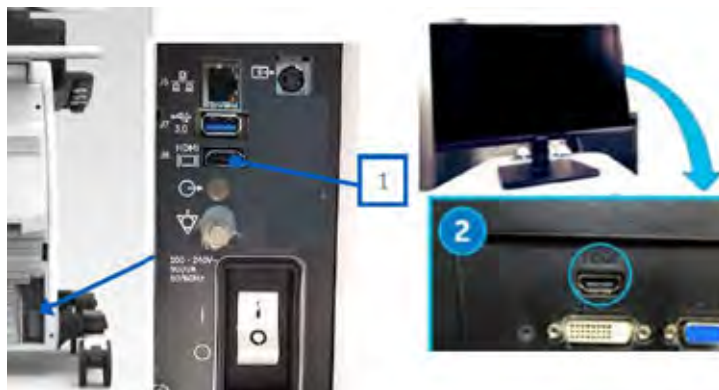
Figure 3-8 Connect HDMI Cable to back of ultrasound system and External Monitor
