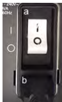
Figure 3-13 Circuit Breaker (a) and Power Plug (b)
