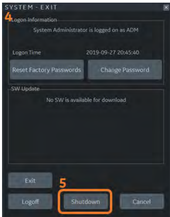
Figure 13-319 Shutdown to Begin Installation
