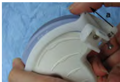
Figure 11-40 Remove the biopsy guide
