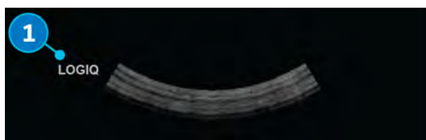
Figure 11-4 Probe orientation marker on the display
