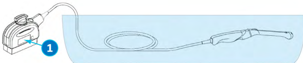
Figure 11-13 Probe Immersion Level for IC5-9-D, E8C, and E8C-RS with serial numbers listed above
