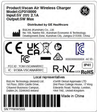
Figure 13-178 Vscan Air CL Model GP310000 and GP320000 Rating Plates
