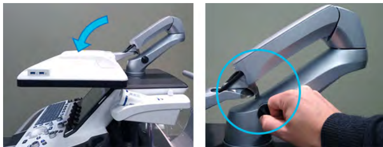
Figure 3-51 Flip down the monitor and lock the monitor arm
