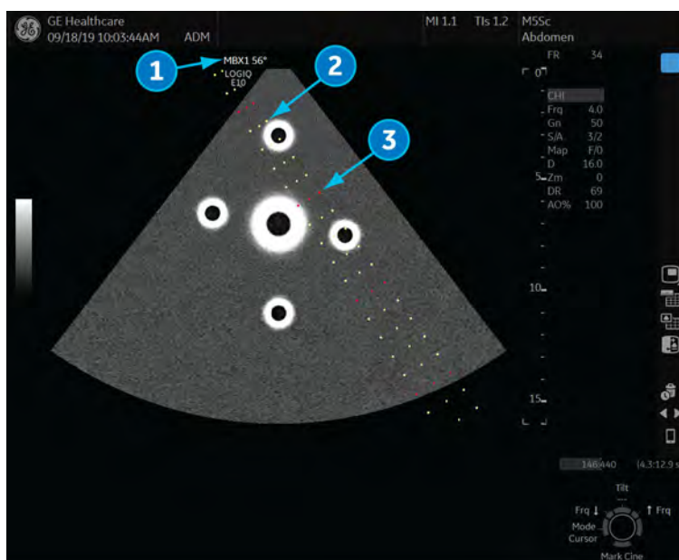
Figure 11-21 Biopsy Guidezones for the M5Sc Probe
