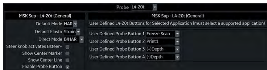
Figure 11-1 Assigning Different Functions to the Probe Buttons
