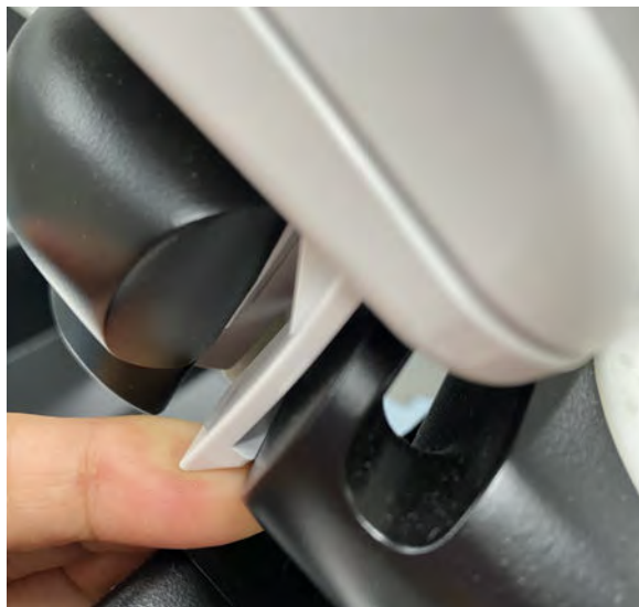
Figure 12-16 Pull the claw to remove
