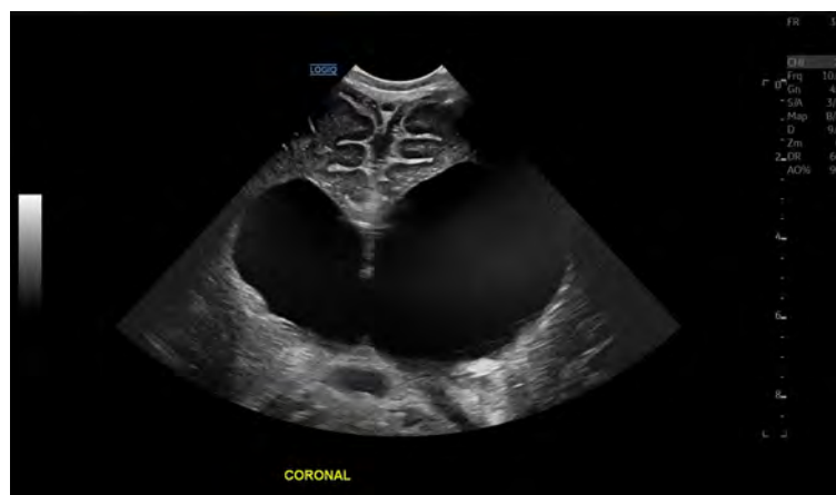
Figure 5-12 Image with Grating Lobe Artifact Removed
