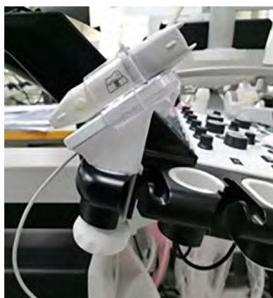
Figure 13-163 Vscan Air On Console Charger Installed (with Probe)
