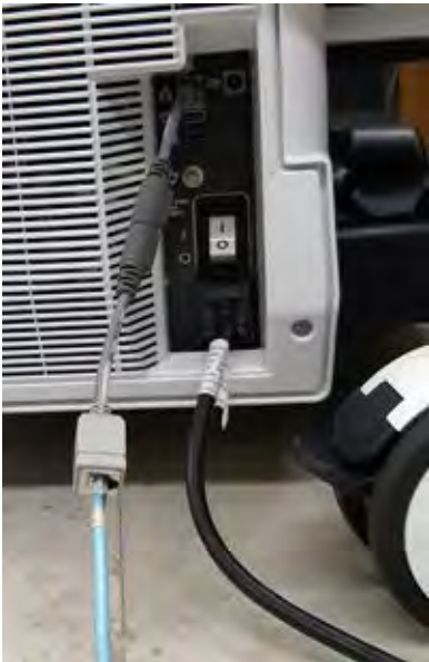
Figure 3-7 LAN Cable with Protection Cable (Example)
