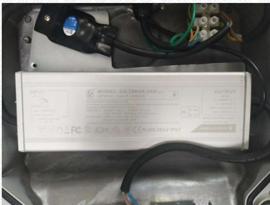
Photo 5: Test result of IP6X and IPX6 test for model RL-S8-200W
