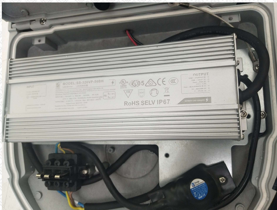
Photo 5: Test result of IP6X and IPX6 test for model RL-S7-320W
