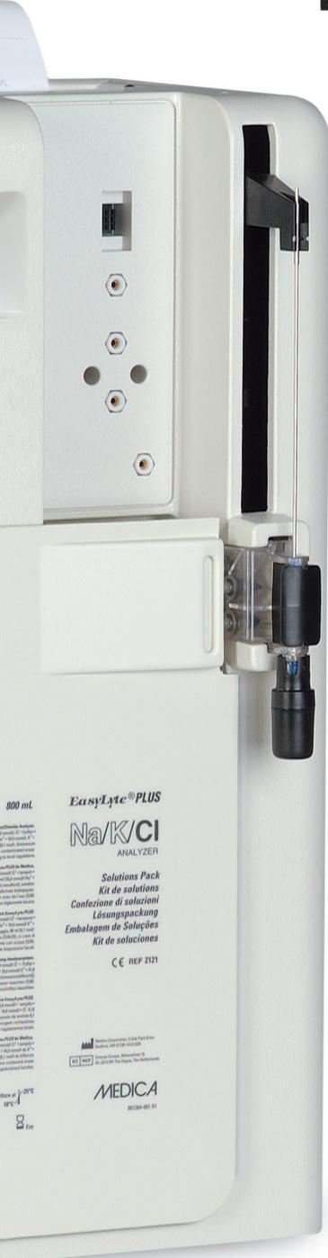
Self-contained Solutions Pack contains liquid calibrants and collects all waste, eliminates sample contact
