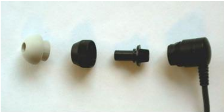
Disassembled OAE probe. Note probe tips after year 2010 are transparent instead of black. As well are ear tips in, e.g., green, blue, red, and yellow colors.
