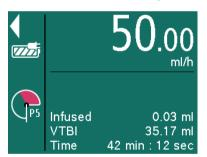
The set pressure level is shown with a P (for pressure) and a number. In addition, a red area shows how quickly the set pressure alarm limit will be reached. The "manometer" display shows the current pressure in the system. The lower the set pressure alarm limit level is, the larger the red area is, the quicker this limit is reached and a pressure alarm triggered.
