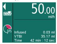
Note: The infusion rate set can be changed during an ongoing infusion by pressing the OK kev.
