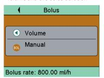
Note: If the bolus administration is not started after the Bolus key is pressed, the device automatically returns to the delivery screen for the ongoing infusion.
