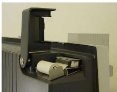
FIGURE 14: INSTALLATION OF PRINTER PAPER
