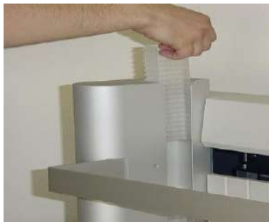
FIGURE 13: INSTALLATION OF CUVETTES
