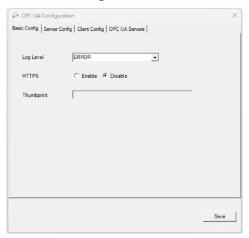
To configure the OPC UA driver, navigate to the *OPC UA*Configuration window in the IoT Driver Configurator. This interface consists of multiple tabs for setting up and managing the OPC UA service.
