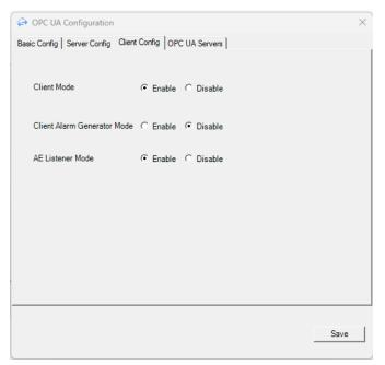
The *Client Config* tab configures the OPC service to act as a *Client* connecting to external OPC UA servers. When in client mode, the OPC service can read values from connected servers and trigger events based on alarm conditions.
