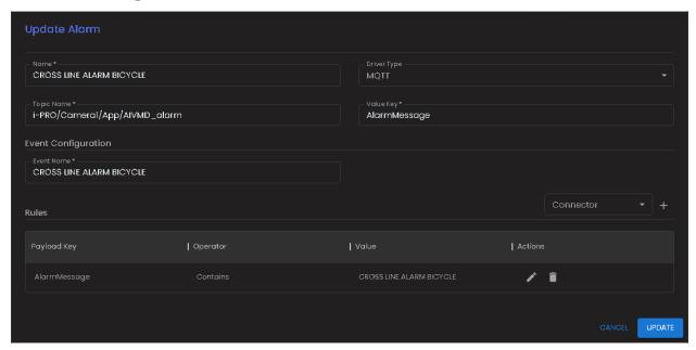
To trigger user-defined events in XProtect upon receiving an alarm payload, follow these steps. It's important to first configure the corresponding alarm within the XProtect Management Client to ensure proper functionality.
