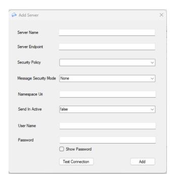
After entering the necessary details, use the *Test Connection* button to verify connectivity. Once confirmed, click *Add* to save the server configuration. The added server will now be listed as an option in the *OPC Server* dropdown within the *Add Point* window.
