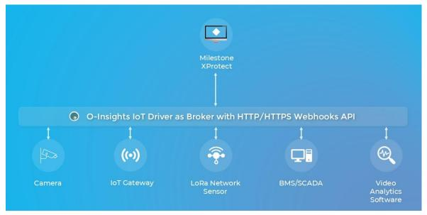
O-Insights IoT Driver can also function as an MQTT broker, managing point data exchange between clients within the O-Insights MQTT broker configuration.
