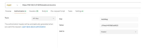
After all required configurations have been performed, click on *Save*. Restart the MQTT driver to apply changes.
