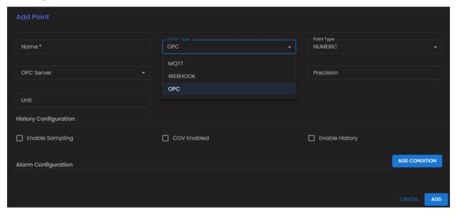
To add an OPC point, use the *Add Point* window and select *OPC* as the driver type. Here, users can set up point configurations:
