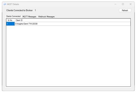
Clients Connected: Shows all the connected clients to the MQTT broker.
