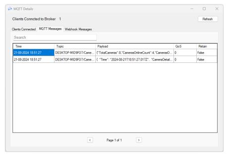
MQTT Messages: Displays every topic received by the MQTT broker, containing information sent by MQTT clients.
