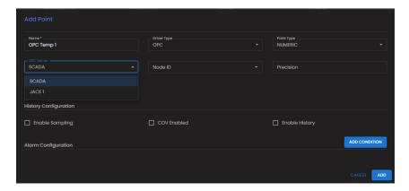
Node ID: Choose or enter the Node ID for the OPC point. For example, if connecting to SCADA, select a node from the server's list of exposed nodes. NodeIDs will be filtered based on their PointType.
