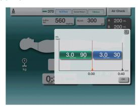
Thumbnail style display – Quickly view injection time and volume and confirm protocol settings visually.
