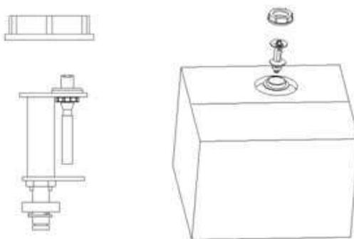
Figure 2-5 Installation of waste liquid level sensor
