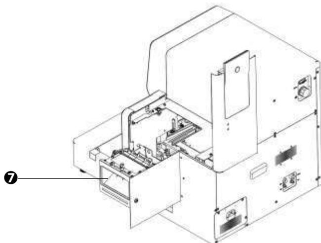
Figure 14-4 Clean the strip-transport plate - step 3
