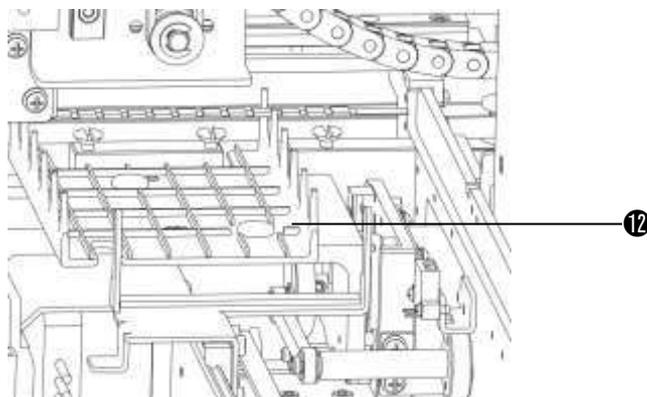
Figure 14-6 Clean the strip-transport plate - step 5
