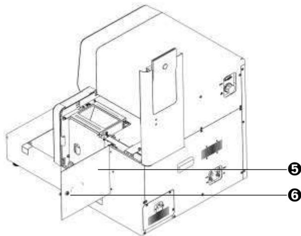
Figure 14-3 Clean the strip-transport plate - step 2
