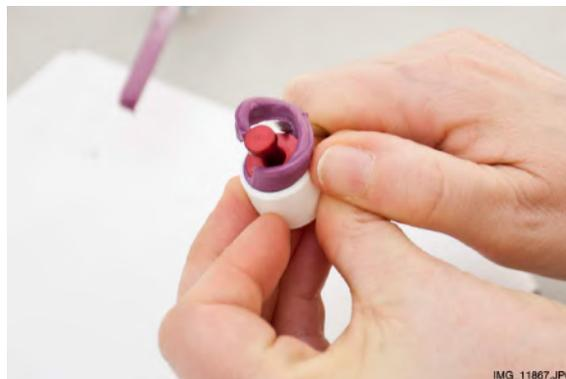
5. Gently pull the calibration pin out and ensure that the surfaces of the hole formed by the calibration pin are even (no air bubbles in inside walls).
