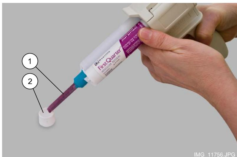
2. Place the calibration pin provided (part number 10031265) in the material.
