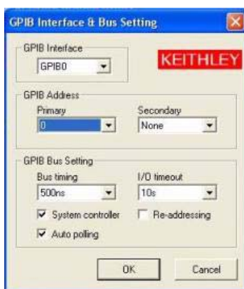
Figure 12: GPIB interface and bus configuration
