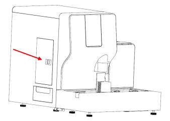
Figure 14-7 Cleaning sheath fluid bottle
