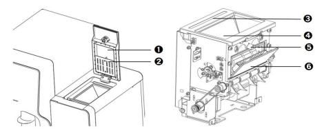
Figure 5-1 Strip and desiccant placement illustration
