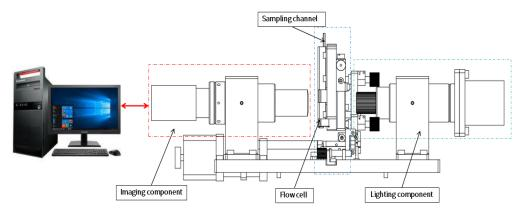
Figure 4-1 Schematic diagram of imaging principle
