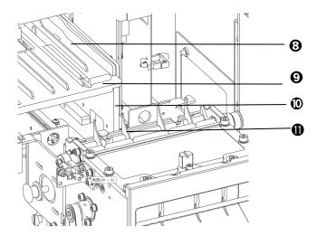
Figure 14-5 Clean the strip-transport plate - step 4
