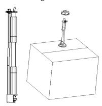
Figure 2-4 Installation of sheath fluid sensor
