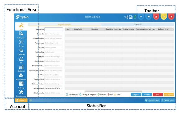
Figure 3-5 Operation interface of software
