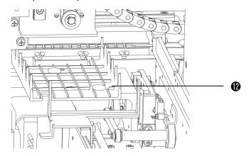
Figure 14-6 Clean the strip-transport plate - step 5
