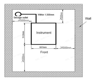
Figure 2-1 Space requirements for installation
