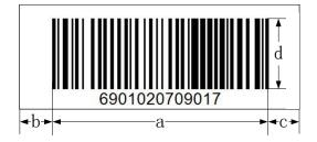
Figure 5-2 Barcode specifications illustration
