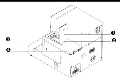
Figure 14-2 Clean the strip-transport plate - step 1
