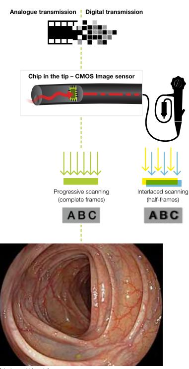
The CMOS chip is positioned directly in the tip of the endoscope and transforms the analogue signal into a digital signal at the site of examination. This ensures brilliant image transmission with reduced noise.
