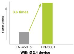
The 3.2 mm working channel provides greater suction performance than conventional models.\*
