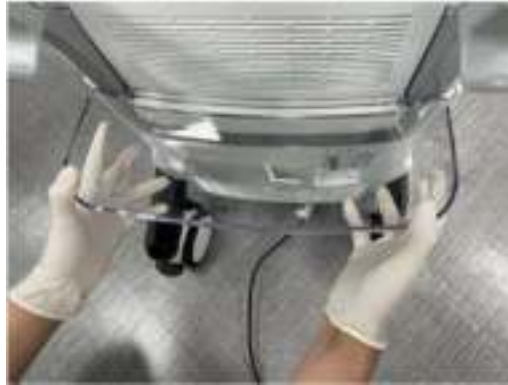
Figure 12-15. Disassemble the rear basket
