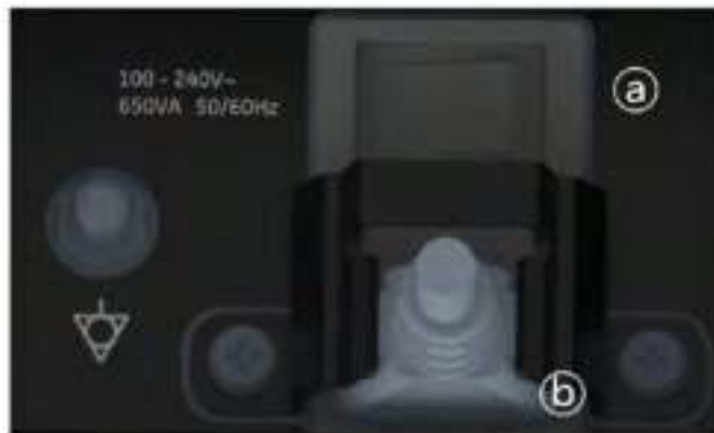
Figure 3-8. Circuit Breaker (a) and Power Plug (b)
