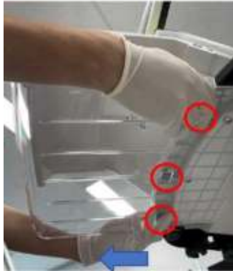
Figure 12-14. Disassemble the Control panel rear tray
