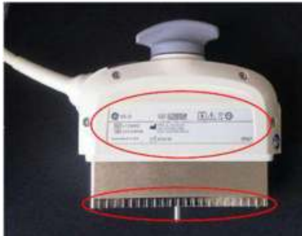
Figure 11-8. Connector/console interface surface and label
