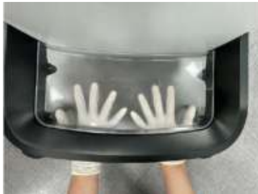
Figure 12-13. Disassemble the base tray
