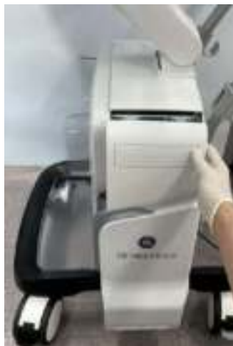
Figure 12-11. Remove the side cover left or right
