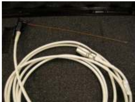
Figure 13-132. Needle Tip Sensor and Cable Close-up
