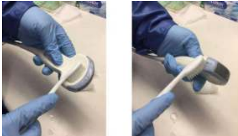
Figure 11-6. Cleaning the probe using a brush
