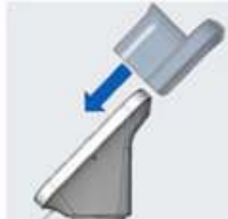
Figure 13-185. Install Probe Holder on Charger
