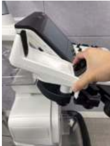
Figure 3-4. Install TVTR Probe holder
