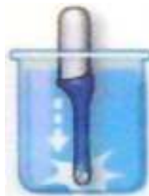
Figure 11-13. Probe suspended in disinfectant basin
