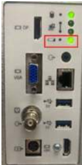
Figure 13-303. LED location of the battery
