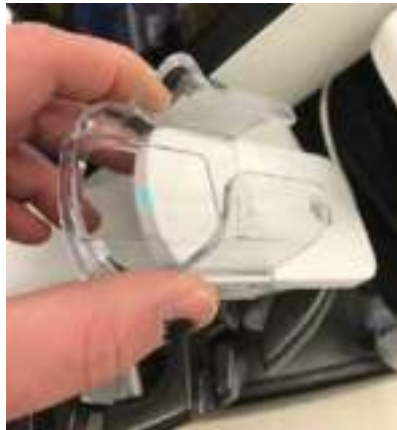
Figure 13-200. Remove Vscan Air Probe Holder
