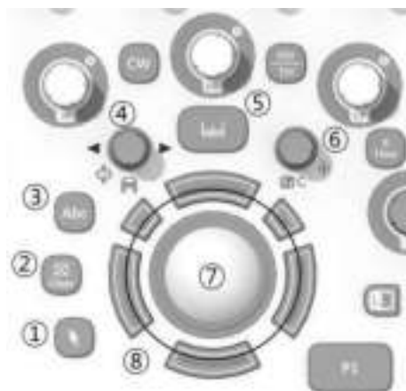
Figure 7-3. Measurement Controls on the Control panel
