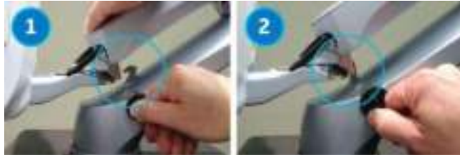
Figure 3-35. Unlock/Lock the monitor arm
