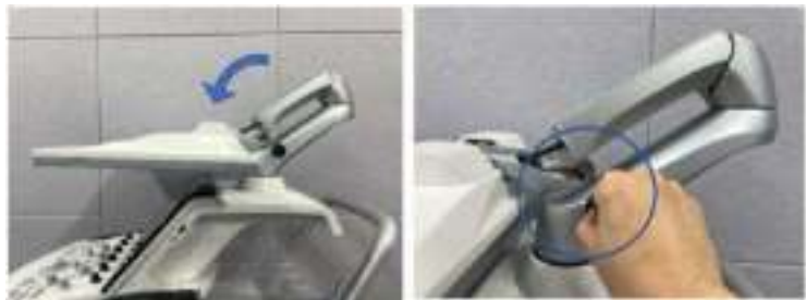
Figure 3-40. Flip down the monitor and lock the monitor arm
