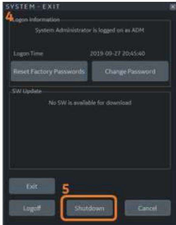
Figure 13-274. Shutdown to Begin Installation
