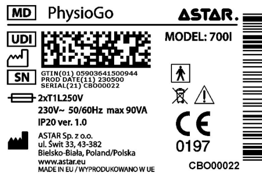
Figure 4.8. Name plate of PhysioGo device – version 1.0
