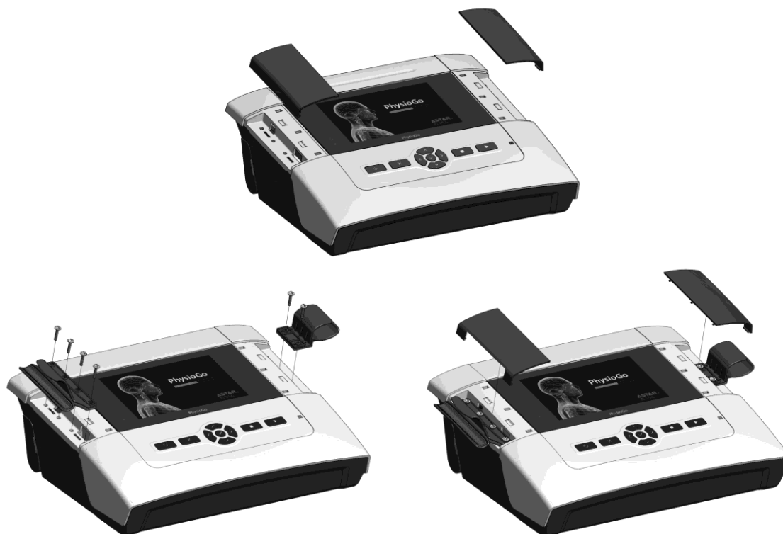
Figure 4.5. Sample view of mounting the holders for point laser applicator and ultrasound head
